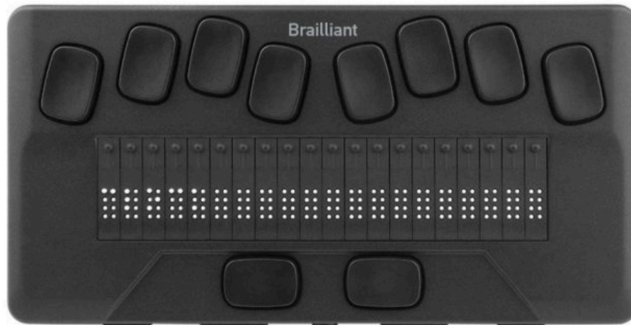
Figure 2: Top Face View of Brailliant Device (Humanware, 2024).
